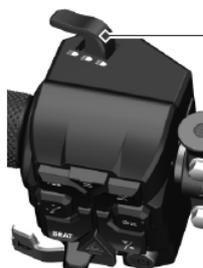
**High and low beam overtaking light buttons**
